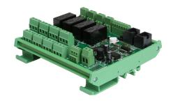
The ARU104MK2 is an intelligent relay unit featuring four double pole relays with normal open and normal closed contacts. Control can be done through both digital (RS-485) and analogue (contact) input signals. Thanks to the flexible structure in terms of connectivity and control, the ARU104MK2 can be implemented in a wide variation of applications, adding flexible and intelligent functionality to your audio & video related or any other project.
